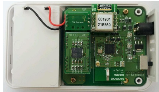
Figure 2. Assembled Extension Board with 3 sensing modules
