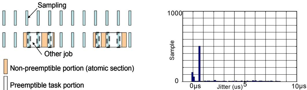
FIGURE 3: (a) Occurrence of Jitter, (b) Histogram of Jitter at 5KHz
