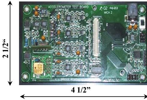
FIGURE 1. Sensor Board with 4 Accelerometer Channels
