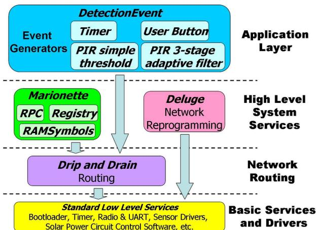
Fig. 3. Software services on the sensor network platform. The core network management services are *Deluge* for network reprogramming [7] and *Marionette* for fast reconfiguration of parameters on the nodes [8]. The *DetectionEvent* application relies on the *Drip and Drain* routing layer for dissemination of commands and collection of data [9]. For more details on the software architecture used in the outdoor testbed, see [3], [8].
